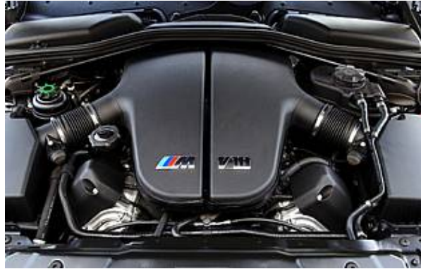
Monstrous 5.0-litre V10 engine packs an incredible 507bhp punch
